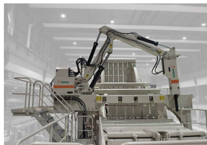
Figure 10. New crushing hammer on the first in the technological chain sieving screen (METSO [64]).
